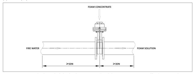
Note: Foam pressure must be 1 bar to 2 bar higher than the water pressure through the proportioner. A minimum of five diameters straight pipe is required upstream and three diameters straight pipe is required downstream.
